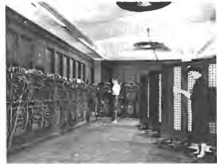
Figure 20N.1 ENIAC: the first US fully electronic computer (US army photo).
