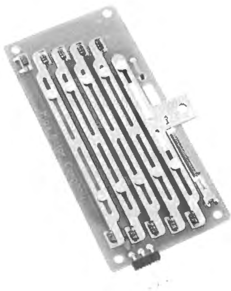
Figure 26N.30 MigaOne amplifies stroke length for nitinol wire actuator.
