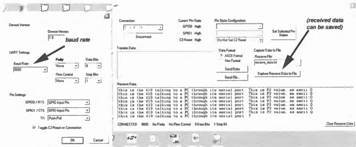
Figure 24L.12 SiLabs terminal screen: UART settings and main window as micro talks to PC through UART.
