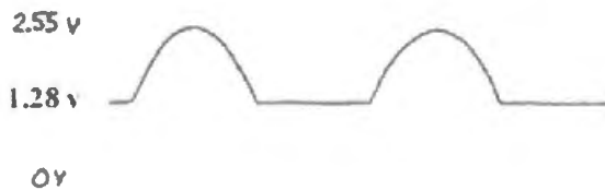
Figure 23N.13 Half-wave rectification centered about waveform midpoint.
