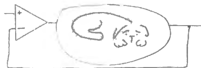
Figure 9N.8 Something with slow response, inside loop, can cause trouble.
