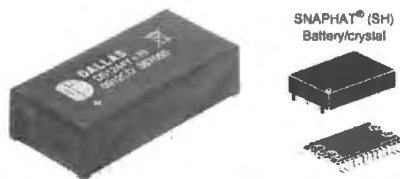
Figure 17N.5 Chubby RAM acts like RAM, but remembers for 10 years. Figure used with permission of Dallas/Maxim.
