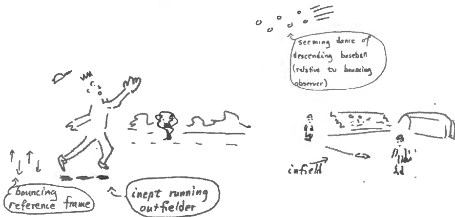
Figure 8N.7 Baseball dances the way comparator input dances – once the outfielder's reference frame starts jumping.
