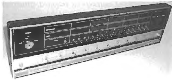
Figure 20N.7 Front panel of a Data General Nova computer (born 1969).
