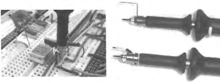
Figure 20L.14 A minimal ground lead minimizes ringing.
