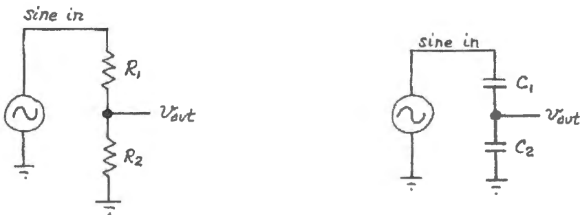
Figure 2N.16 Two dividers that deliver 1/2 of V_{in} – with no phase shift.
