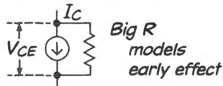
Figure 5S.6 A non-ideal current source can be modelled as ideal parallel (large-) R .
