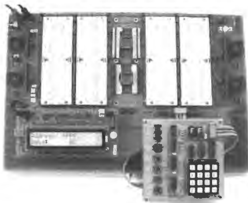
Figure 16L.4 Display and keypad connected to the breadboard.
