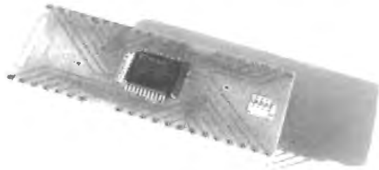
Figure 16L.6 PAL (TQFP package) mounted on a carrier, to permit breadboarding.
