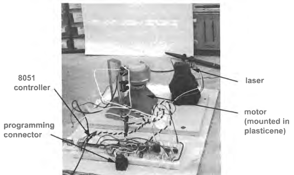
Figure 26N.5 Laser display; showing projection on a sheet of paper (incoherent image, in this photo).
